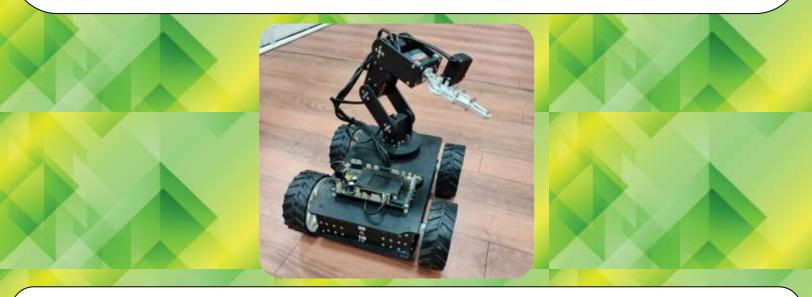
**Basic RoboCar:** Designed for electronics students, this RoboCar does not require a microcontroller to operate. It is equipped with various sensor modules that allow it to sense and react to its environment. Its capabilities include fire sensing, clap sensing, light detection, object following, obstacle avoidance, and more. The RoboCar can be interfaced with microcontrollers for advanced functionality, making it a versatile platform for learning and experimentation.
